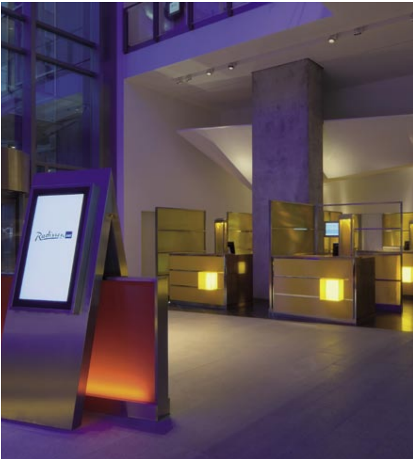
Fig. 3. DALI is used as the basis for flexible light groups and simple configuration of light scenes for an optimum room effect
